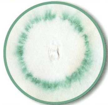
CHLOR 250 / CHLOR S250 / CHLOR S700 Microtracer RF Green Lake Developer: 7% Sodium Carbonate in water
